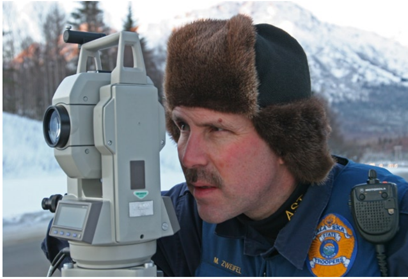
Trooper Mike Zweifel, one of the few troopers certified on Total Station measurements of serious-injury of fatal vehicle crashes, surveys a scene of a fatal crash on the Seward Highway.
