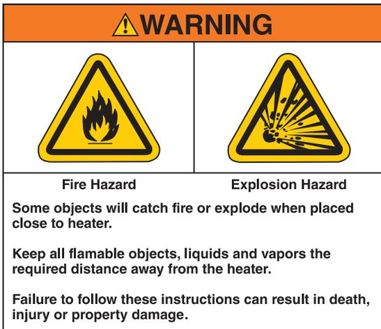
Clearances are the required minimum distances that combustible objects can be placed from the heater to prevent fire hazards. Combustibles are materials which may catch on fire and include common items such as wood, paper, rubber and fabric. Clearances to combustibles must be maintained at all times to ensure safety.
