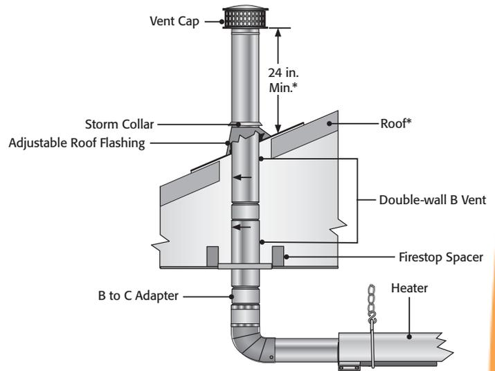
\*Consult the NFPA 54/ANSI Z223.1 or CAN/CSA-B149.1 Gas Vent Termination criteria if roof pitch exceeds 9:12 and refer to manufacturer's installation instructions for vent size and length.
