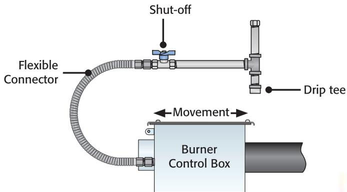
Connect heater to gas supply using the proper equipment as set forth by ANSI standards, NFPA codes and the manufacturer. Consult manual for instructions on pressure, expansion and other safety requirements; including local codes.
