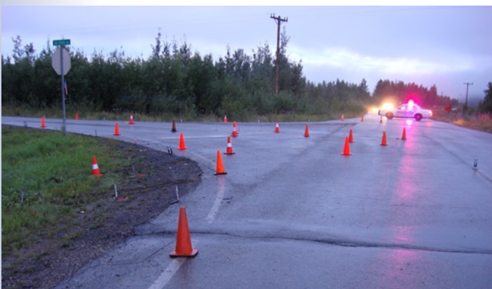
Cones mark the distance between measurements to use in Photogrammetry.
