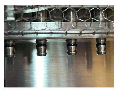
Rings that appear shiny and sufficiently lubricated (as shown in this image) do not require additional greasing.
