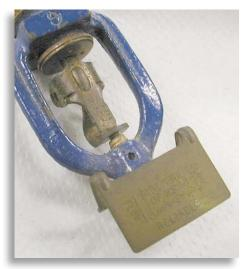
The blue frame on this sidewall sprinkler indicates its fusible element has an operating temperature range of (250 to  $300 \degree F [121 to 149 \degree C]$ ) ranking it in the "high temperature" category.
